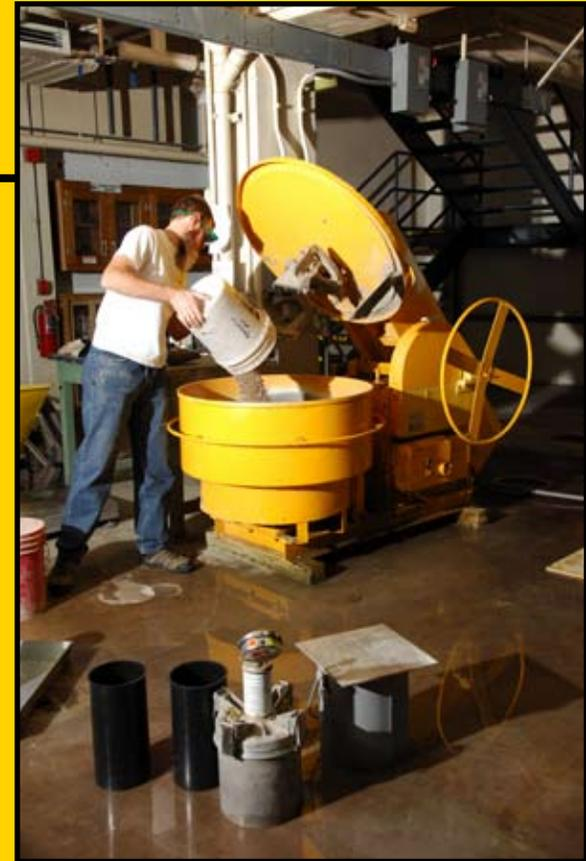
Benedict laboratory provides 15,000 ft<sup>2</sup> for concrete mixing, curing and testing. MS student Paul Koning is shown above preparing a batch of concrete for testing.
