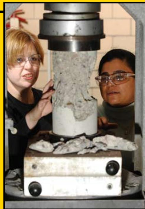
MS student Corrie Craft and Dr. Yogini Deshpande examine a concrete specimen that failed a compression test.
